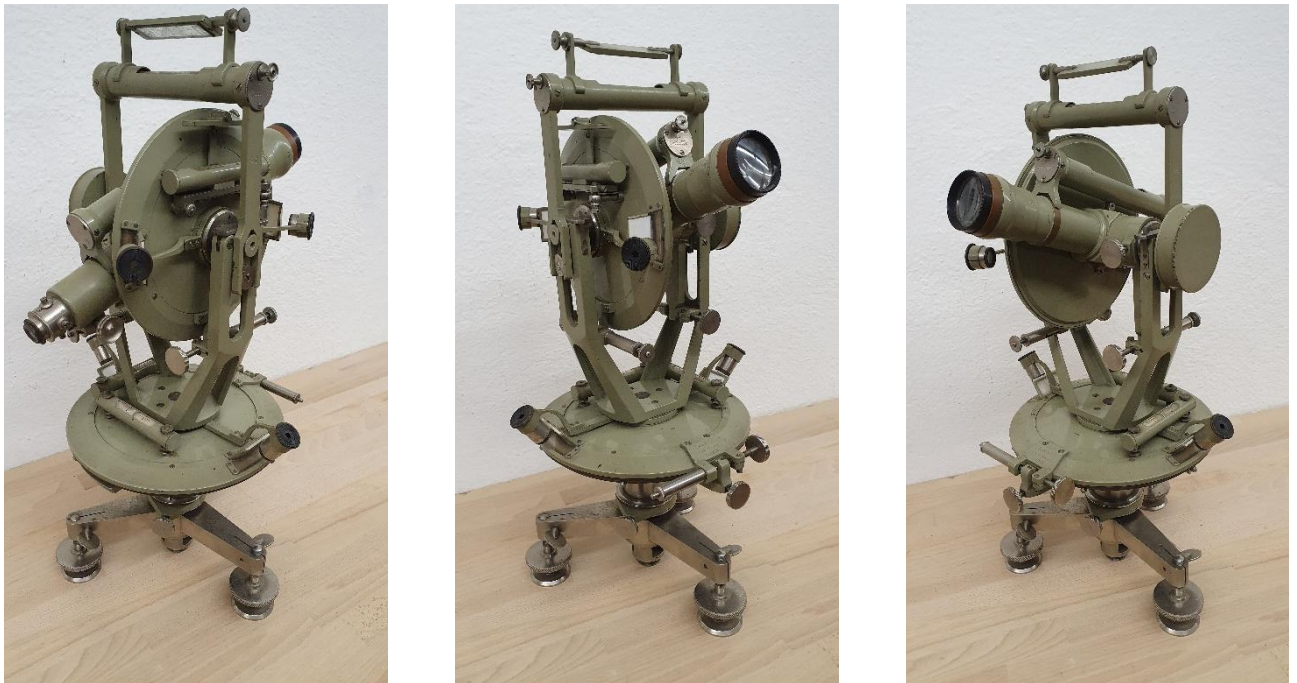
Abb. 12, 13, 14: Passage-Instrument Modell Kern, Nr. 19114 (Lardelli 1907)
